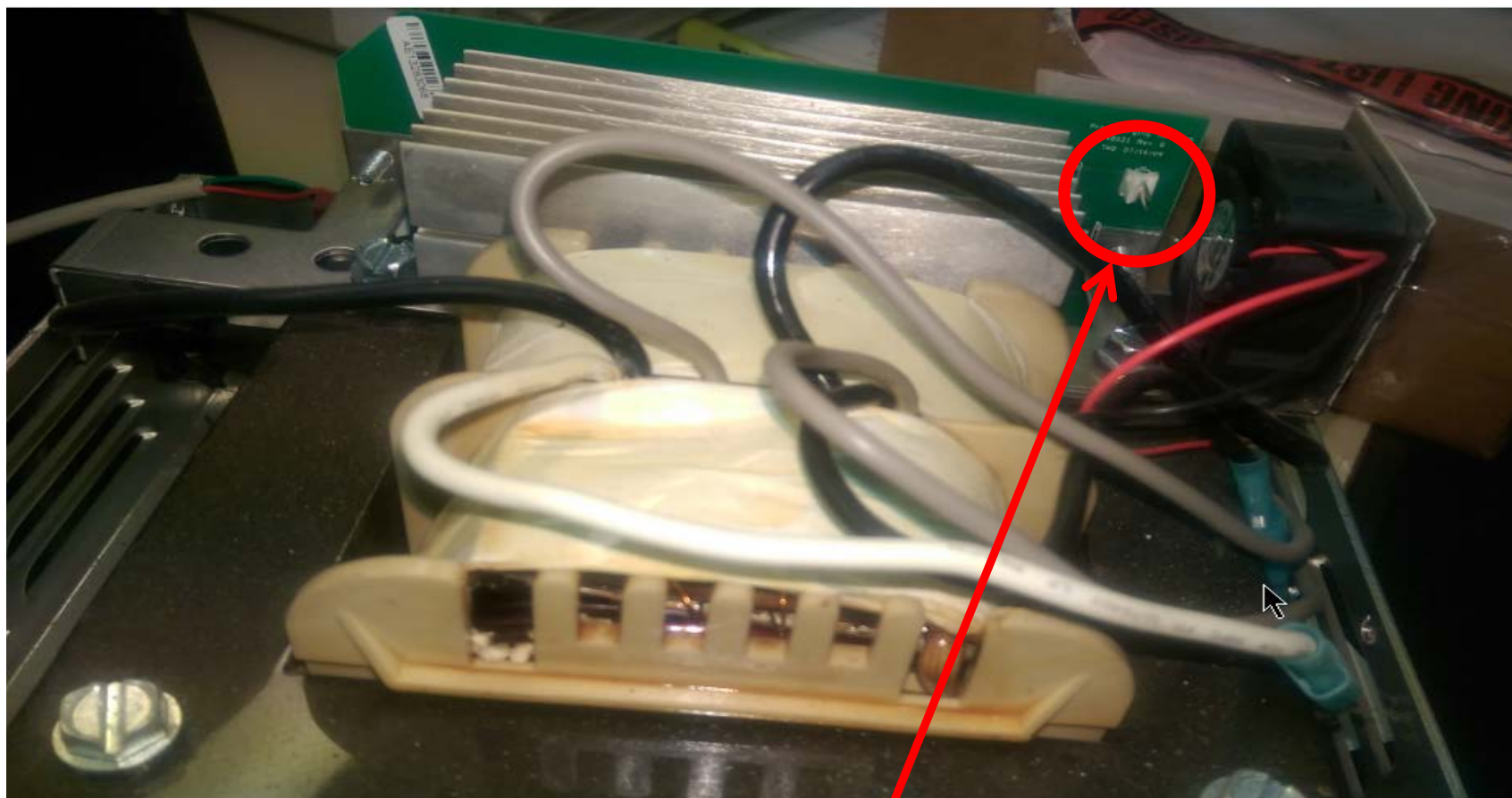
Charger is set for wet cell, jumper is off of pins.
